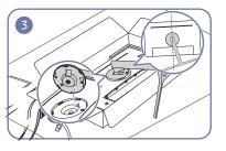
Place the stand neck of the display on the device as Stand assembly is complete. per the positions of the fasteners.
