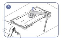
counterclockwise for 10°, lift the stand neck to detach it from the device.
