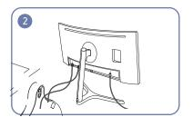
Connect cables to the appropriate ports.
