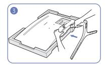
Place the protective Styrofoam (cushion) included in the package on the floor and place the product facing down on the Styrofoam, as shown in the image. If Styrofoam is unavailable, use a thick sitting mat. Hold the back of the monitor as shown in the figure. Push the assembled stand into the main body in the direction of the arrow as shown in the figure.
