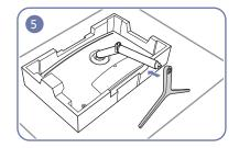
Insert the stand base into the stand neck in the direction shown in the figure.
