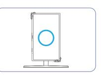
• When moving the monitor, rotate to portrait orientation and hold the top and bottom of the monitor.
