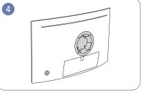
A Attach the BRACKET WALL here
