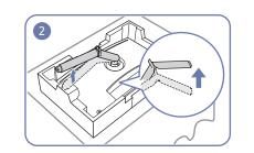
While pressing down with one hand on the lower styrofoam layer, lift the stand's neck with the other hand.
