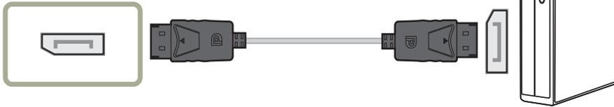
— A DP cable shorter under 1.5 m in length is recommended. Using a cable longer than 1.5 m can affect the picture quality.
