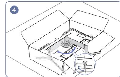
4 Turn the stand neck of the display clockwise for 90° to ensure that the stand neck of the display is put into place.
