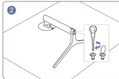
2 Check that the stand neck is firmly connected. Tightly fasten the connecting screw at the bottom of the stand base.
