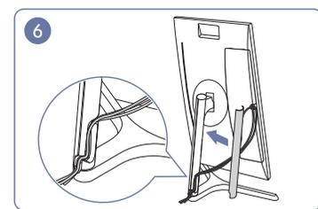
6 Place the corresponding cables into the stand-neck holder. Do not stretch the line. Three cables in one holder is recommended.
