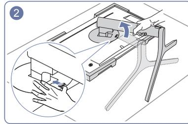
Push the key upward and hold. Turn the stand neck of the display counterclockwise for 10°.
