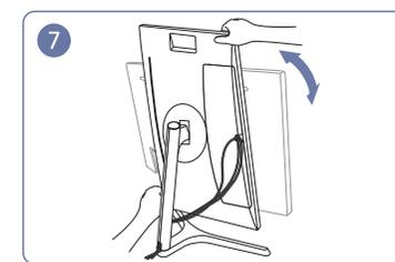
7 Rotate the machine to the horizontal position.
