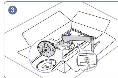
3 Place the stand neck of the display on the device as per the positions of the fasteners.
