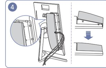
4 Arrange the cables through the groove on the COVER-REAR, and then attach the COVER-REAR SUB. When you attach the COVER-REAR SUB, please aim six ribs of the COVER-REAR SUB to the bottom holes of the COVER-REAR at first.
