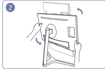
2 Rotate the machine to the highest vertical position.
