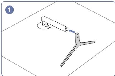
1 Insert the stand neck into the stand base in the direction shown in the figure.
