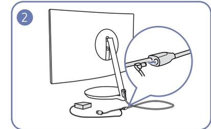
Connect the AC/DC adapter cable to the DC 19V port of HDMI (+DC JACK) cable.
