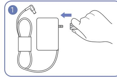
Connect the power plug to the AC/DC adapter.
