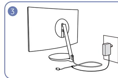
Plug the AC/DC adapter into the power outlet.
