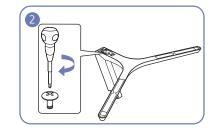
Tightly fasten the connecting screw at the bottom of the stand base.
