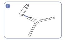
Insert the stand neck into the stand base in the direction shown in the figure. Check that the stand neck is firmly connected.
