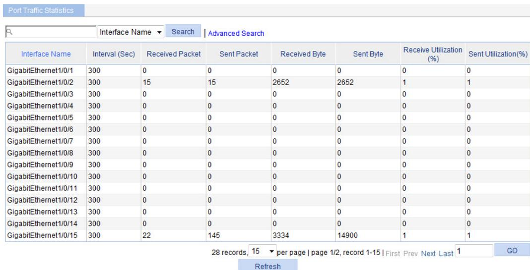
The screenshot shows the 'Port Traffic Statistics' interface. At the top, there is a search bar with 'Interface Name' and a 'Search' button. Below the search bar is a table with the following columns: Interface Name, Interval (Sec), Received Packet, Sent Packet, Received Byte, Sent Byte, Receive Utilization (%), and Sent Utilization(%). The table lists 15 GigabitEthernet interfaces (GigabitEthernet1/0/1 to 1/0/15). The data for each interface is as follows:
