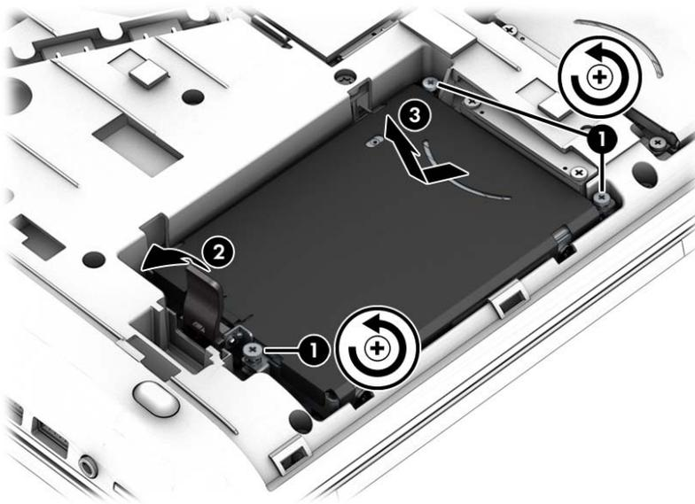
7. Lift the hard drive (3), and then pull the hard drive out of the hard drive bay.
