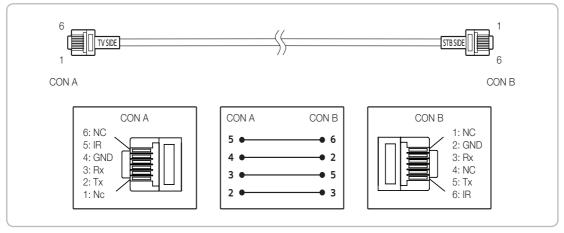
Operation Specification of Data Cable(RJ12): RS232
