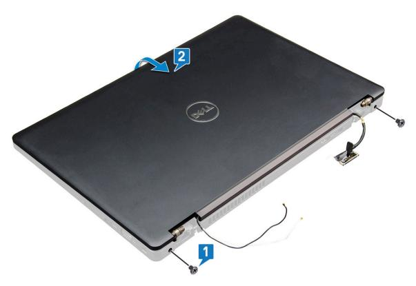
Slide upward the display assembly away from the system base.
