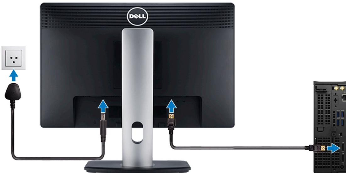
**i** **NOTE:** If you ordered the computer with a discrete graphics card, the HDMI and the display ports on the back panel of the computer are covered. Connect the display to the discrete graphics card.
