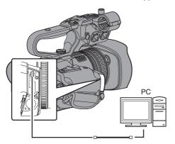
2 Select [Change] using the cross-shaped button (▲▼), and press the Set button (♠). The camera recorder switches to USB mode.
