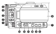
1 [FULL AUTO] Full Auto Selection Button Press and hold the button to switch the Full Auto mode ON and OFF. Full Auto mode adjusts the Iris, Gain, Shutter
