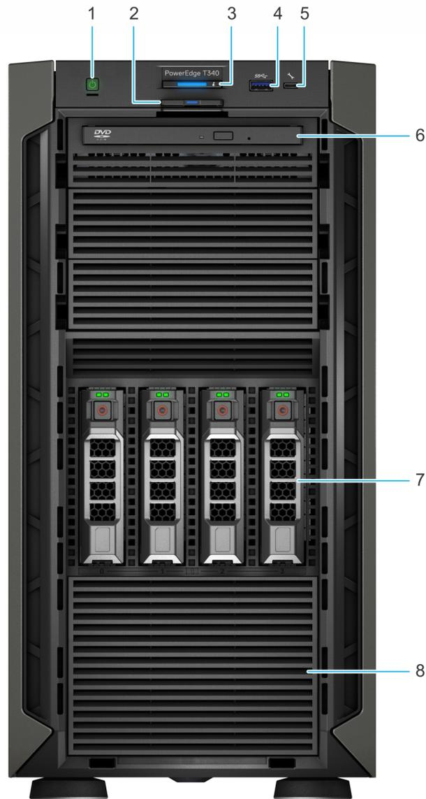
**Figure 2. Front view of 4 x 3.5-inch drive system**
