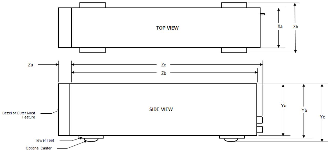
Figure 5. Chassis dimensions
