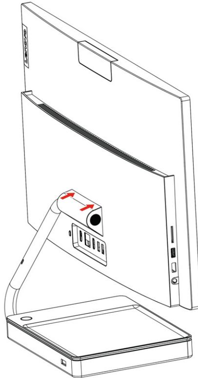
7. Reconnect the ac power adapter and all disconnected cables to the computer.
