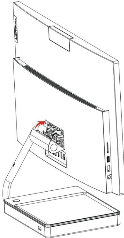
6. Slightly press the hinge cover until it snaps into position.
