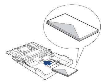
5. Gently press and slide the paper width guides (1) and paper length guide (2) to fit the size of the envelopes. Make sure the envelopes are flat in the tray.
