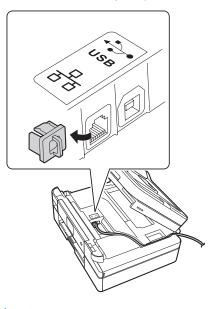
Carefully guide the cable through the cable channel and out the back of the machine.
