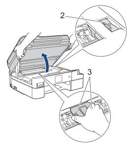
• If the paper is jammed under the print head, unplug the machine from the power source, and then move the print head to take out the paper.
