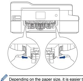
Depending on the paper size, it is easier to remove the jammed paper from the front of the machine rather than from the back of the machine.
