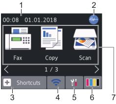
This screen shows the machine's status when the machine is idle. When displayed, it indicates that your machine is ready for the next command.
