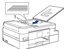
4. Place your document, face down, top edge first in the ADF underneath the paper guides until you feel the document touch the feed rollers and the LCD displays [ADF Ready].
