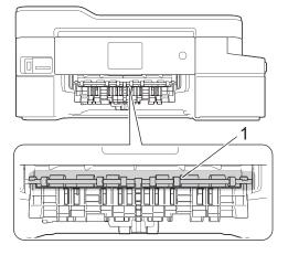
b. Squeeze both levers (1), and then open the Jam Clear Cover at the back of the machine.
