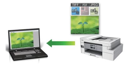
Use the Scan button on the machine to make temporary changes to the scan settings. To make permanent changes, use either ControlCenter4 (Windows<sup>®</sup>) or Brother iPrint&Scan (Mac) software.
