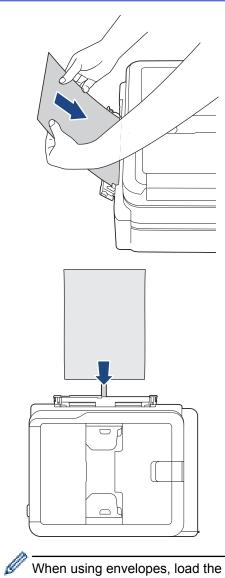
When using envelopes, load the envelopes with the printing surface **face up** and the flap on the left as shown in the illustration.
