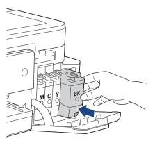
The machine automatically resets the ink dot counter.
