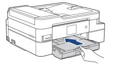
9. While holding the paper tray in the machine, pull out the paper support (1) until it locks into place, and then unfold the paper support flap (2).
