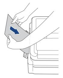
When loading an envelope, or a sheet of thick paper, push the envelope into the manual feed slot until you feel the paper feed rollers pull it.
