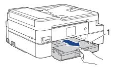
3. Pull the two green levers inside the machine to release the jammed paper.
