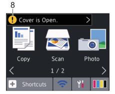
The warning icon **!** appears when there is an error or maintenance message; press **!** to view the details, and then press **X** to return to the Home screen.
