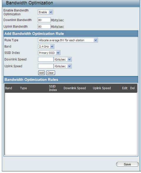
Band: Use the drop-down menu to toggle the wireless band between 2.4GHz and 5GHz.
