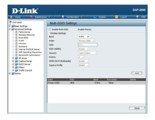
**Encryption:** When you select Open System, toggle between Enable and Disable. If Enable is selected, the Key Type, Key Size, Key Index
