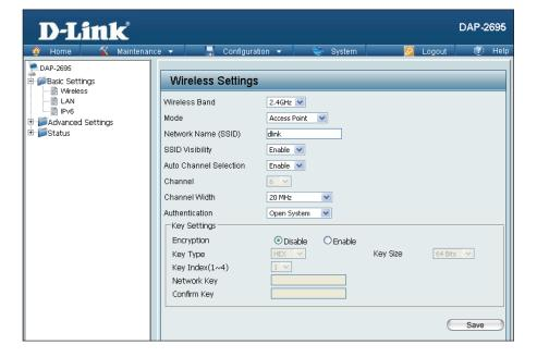
**Channel:** To change the channel, first toggle the *Auto Channel Selection* setting to **Disable**, and then use the drop-down menu to make the desired selection.
