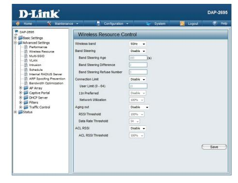
User Limit: Set the maximum amount of users that are allowed access (zero to 64 users) to the device using the specified wireless
