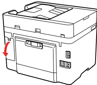
4. Grasp the maintenance box as shown and pull it out of its holder.
