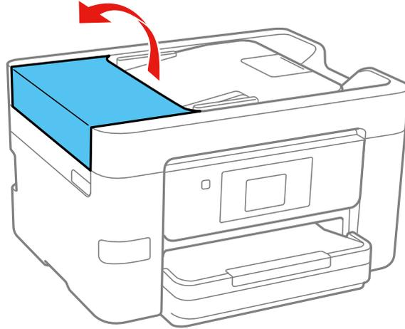
9. Use a soft, dry, lint-free cloth (microfiber is recommended) to clean the rollers and the interior of the ADF.
