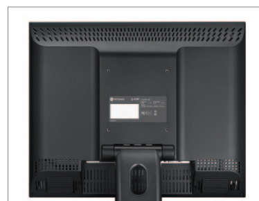
VESA standard wall mount allows for secure mounting
