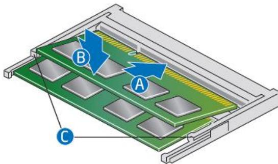
4. Align the small space at the bottom edge of the memory module with the key in the socket.
