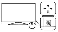
To access the OSD menu on this Philips Display simply use the single toggle button on the backside of the Display bezel. The single button operates like a joystick. To move the cursor, simply toggle the button in four directions. Press the button to select desired option.
