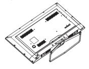
2. Loosen the assembly screws, then detach the neck from the Display.
