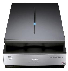
Featuring enhanced high-pass optics that deliver the highest level of image quality with faster scan speeds, the V850 Pro can convert a wide range of media and film formats into professional-quality digital images. This high-productivity 6400dpi scanner requires virtually no warm-up time, can remove dust and scratches automatically and includes two sets of highquality film holders.
