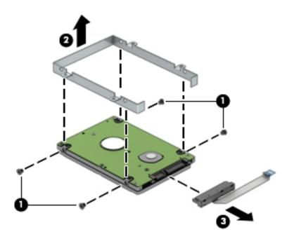
Reverse this procedure to reassemble and install the hard drive.
