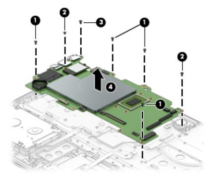
Reverse this procedure to install the system board.
