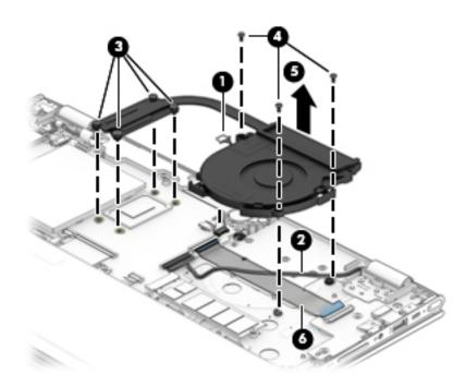
**NOTE:** The thermal material must be thoroughly cleaned from the surfaces of the fan/heat sink assembly and the system board each time the fan/heat sink assembly is removed. Thermal paste is used on the processor (1) and the fan/heat sink assembly section (2) that services it.
