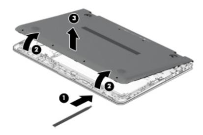
Reverse this procedure to install the bottom cover.
