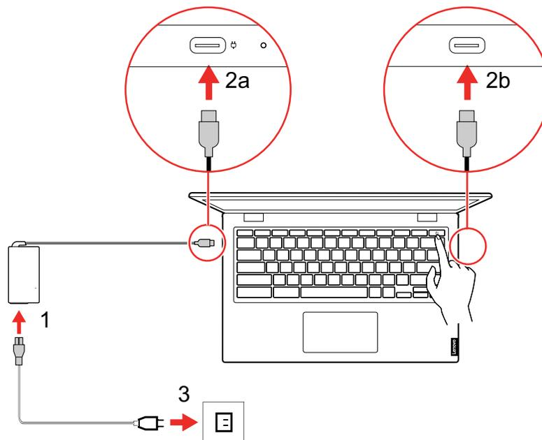
1. Connect the power cord to the ac power adapter.
