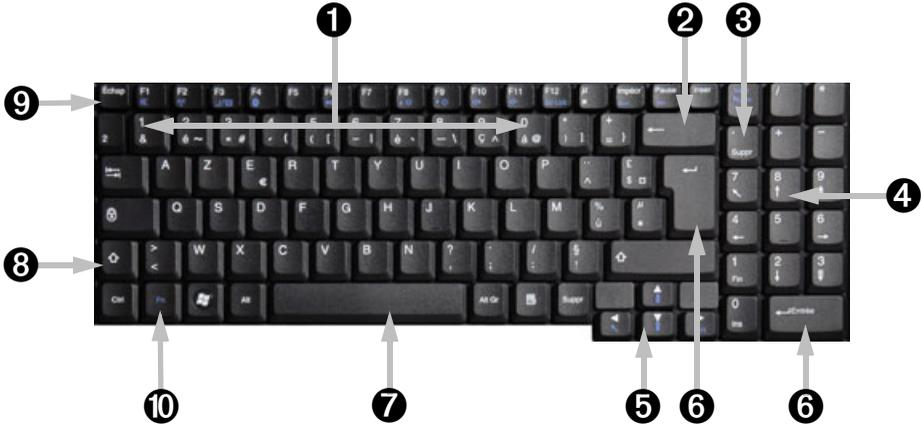
1. **Numbers:** Used to enter numbers and special characters. Press [**Shift**] simultaneously for characters on the top and press [**Ctrl**] + [**Alt**] for characters on the right.
