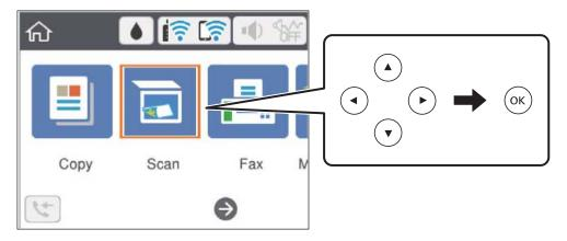
• To change a setting, press the arrow buttons to highlight the setting and press the **OK** button.
