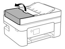
9. Use a soft, lint-free cloth (microfiber is recommended) moistened with a little water to clean the rollers and the interior of the ADF.
