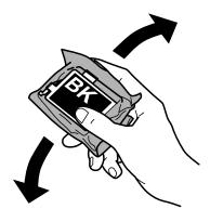
**Caution:** Do not shake the cartridges after opening the packages, or ink may leak.
