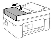
4. Carefully remove any jammed pages from beneath the ADF.
