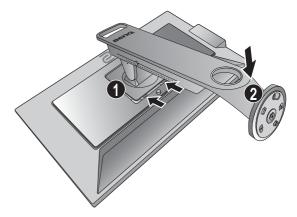
Orient and align the stand base socket with the end of the stand arm. Make sure to align the arrow on the end of the stand to the one on the monitor base.
