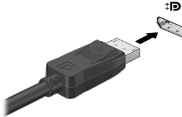
2. Connect the other end of the cable to the digital display device.
