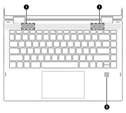
Fingerprint readers can be located on the touchpad, on a side panel of the computer, or on the top cover below the keyboard.
