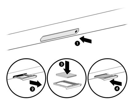
To remove a SIM card, press in on the SIM card, and then remove it from the slot.
