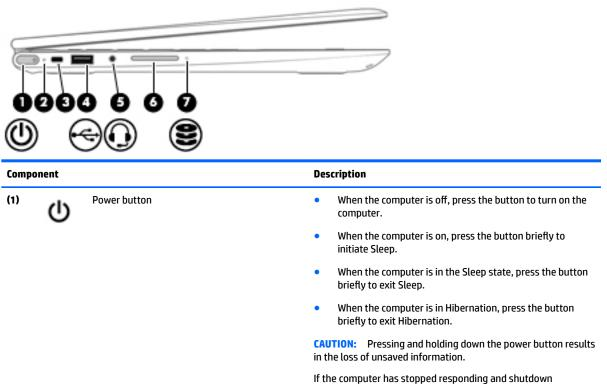
If the computer has stopped responding and shutdown procedures are ineffective, press and hold the power button down for at least 5 seconds to turn off the computer.
