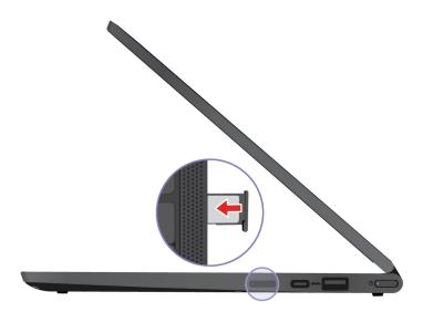
Step 3. Insert the SIM card tray into the SIM card slot.
