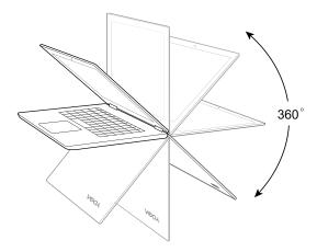
You can switch your display into one of four YOGA modes by rotating the display to a different angle.
