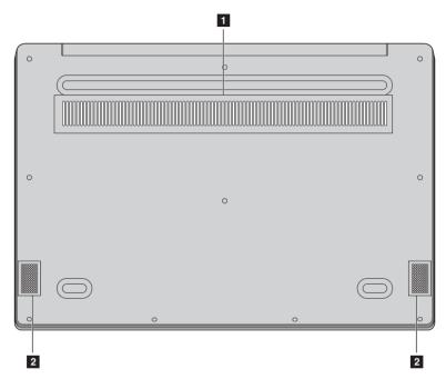
**1 Ventilation slots** Dissipate internal heat.
