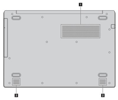
**1 Ventilation slots** Dissipate internal heat.
