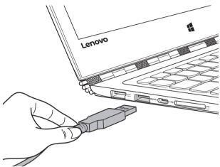
The first time you plug a USB device into a particular USB port on your computer, Windows automatically installs a driver for that device. After the driver has been installed, you can disconnect and reconnect the device without performing any additional steps.
