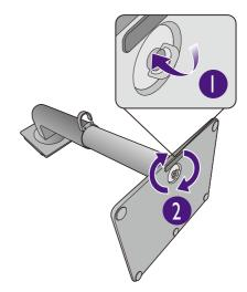
Lift the end of the monitor stand high and orient and align the stand arm with the monitor, then push them together until they click and lock into place.
