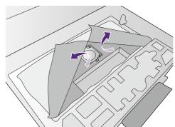
Lift the end of the monitor stand high and orient and align the stand arm with the monitor, then push them together until they click and lock into place.
