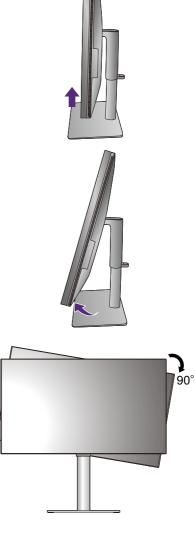
To avoid the edge of the LCD display hitting the monitor base surface while it is being rotated, do tilt and extend the monitor to the highest position before you start to rotate the display. You should also make sure there are no obstacles around the monitor and there is enough room for cables.
