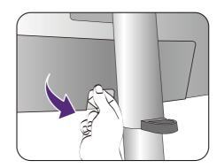
Protect the monitor and screen by clearing a flat open area on your desk and placing a soft item like a towel on the desk for padding, before laying the screen face down on a flat clean padded surface.
