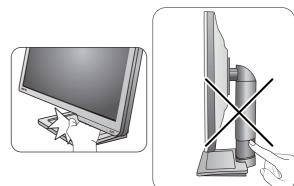
• If the monitor has been rotated to portrait mode and height adjustment is desired, you should be noted that the wide screen will keep the monitor from being lowered to its minimum height.
