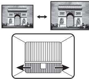
Sharpen the image by rotating the focus ring.
