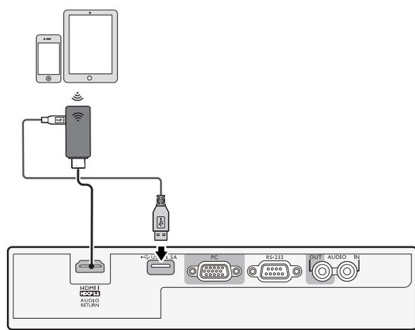
Connect the dongle to **HDMI** and **USB TYPE-A** ports on the projector and switch the input signal to **HDMI 1**.
