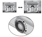
Then sharpen the image by rotating the FOCUS ring.
