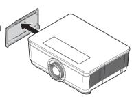
Lift the filter from the filter cover.
