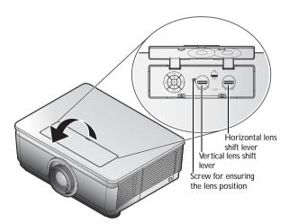
3 Suggest to loosen the screw before lens shift adjustment and tighten up after finished adjustment.
