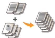
By using Canon PageComposer, you can combine multiple documents into one print job and print the job with specified print settings. This function, for example, enables you to combine documents made with different applications and print all of the pages in the same paper size.
