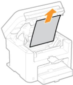
**3** Check whether paper is jammed inside the output guide.
