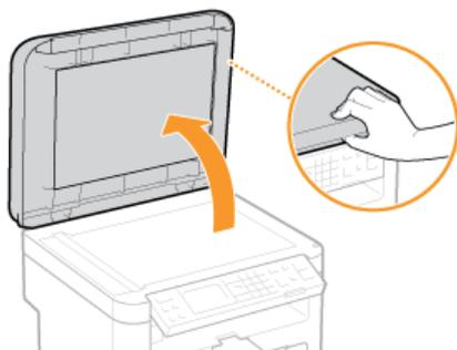
**3 Clean the platen glass and the underside of the platen glass cover.**
