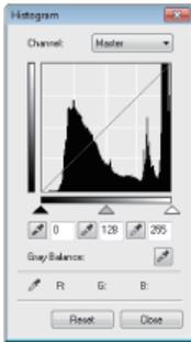
A histogram is a graph that shows the distribution of brightness in an image. You can adjust the image while checking the preview image and histogram. Specify the part of the image you want to make brightest (or darkest) in the preview image, so that the brightness balance of the original image is automatically adjusted with the specified part being the average. Likewise, you can also adjust the balance with the brightness of the medium tone being the average.
