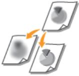
You can adjust sharpness of the copied image. Increase the sharpness to sharpen blurred text and lines, or decrease the sharpness to improve the appearance of magazine photos.
