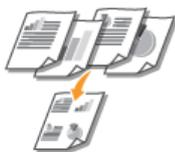
You can print multiple pages onto a single sheet. For example, you can print four or nine pages onto a single sheet by using [4 on 1] or [9 on 1]. Use this function if you want to save paper or to view your document in thumbnails.
