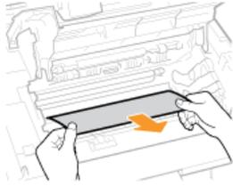
**5** Check whether paper is jammed in the manual feed slot or paper drawer.
