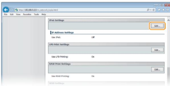
**5** Select the [Use IPv6] check box and configure the required settings.
