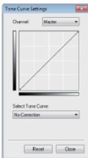
The tone curve is a curved line that indicates the brightness and contrast levels of the image before and after adjustment. Select a registered tone curve to adjust the brightness and contrast levels of the image.
