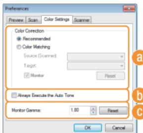
Configure advanced color and brightness settings, such as color matching and gamma correction.
