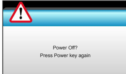
3. Press the "⏻" again to confirm, otherwise the message will disappear after 15 seconds. When you press the "⏻" button for the second time, the projector will shut down.
