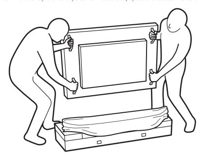
• Do not touch the screen of display. Please use the handles • Keep vertical direction when moving the display. to move the display.
