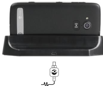
1. Insert the small end
