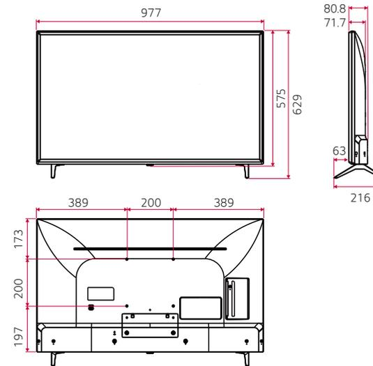
\* UU640C (EU/CIS) series basically have a two-pole stand, but it is able to detach the stand from the body, per service environment (can be used as a wall-mount unit).
