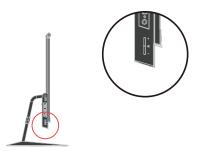
13. When you connect your computer with TYPE-C cable, you can press the USB switch button and follow the OSD menu to chose the USB2.0 with 4K2K picture or USB3.0 with FHD picture.
