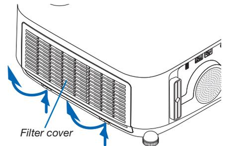
**2. Pick the center of the filter unit for pulling it out.**
