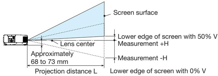
(Note) Height from lens center to lower edge of screen (with tilt feet screwed in)
