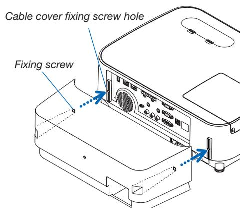
2. **Tighten the cable cover screws.**
