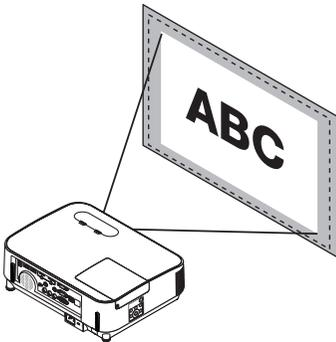
Adjusting the throw angle (the height of an image) [Tilt foot]
