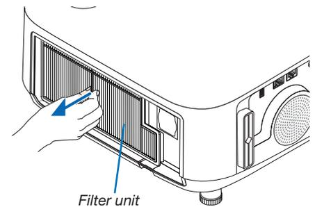
**3. Vacuum dust on the front and back faces of the filter unit.**
