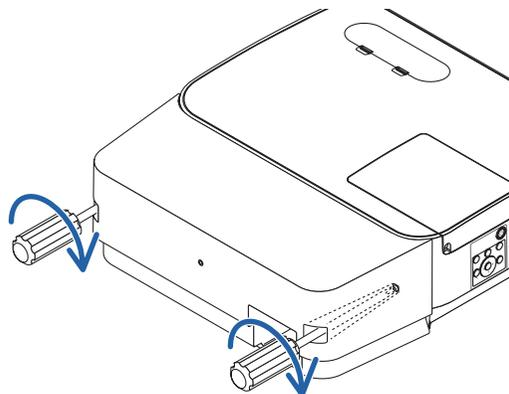
**Removing the cable cover**
