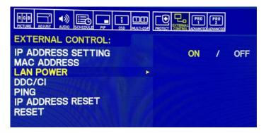
Note that LAN power is OFF out of the box so this will need to be changed for each display within the wall.
