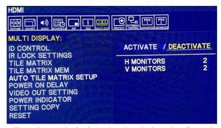
Note that you will need to set the horizontal and vertical monitor dimensions before you activate the Auto Tile Matrix. If done correctly and the LAN is daisy chained as shown on the picture on the previous screen, the displays will automatically adjust so one large picture fills the entirety of the wall. Activating Auto Tile Matrix changes the Tile Matrix, Tile Matrix Mem, Input Signal, Video Out Setting and DisplayPort in the Terminal Settings menu.
