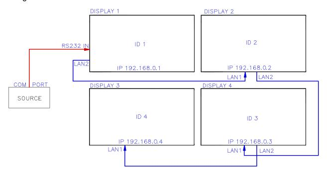
Note that a unique IP address is not necessary to communicate to all displays if display 1 is not connected to a network. The displays will automatically assign themselves IP addresses if no DNS is detected and the IP Setting within the IP Address Setting in the External Control menu is set to AUTO. Note that this is the setting out of the box.
