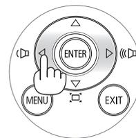
**TIP:** The [BEEP] sound volume cannot be adjusted. To turn off the [BEEP] sound, from the menu, select [SETUP] → [OPTIONS (1)] → [BEEP] → [OFF].
