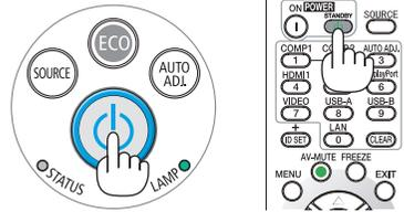
2. Secondly, press the ENTER button or press the
