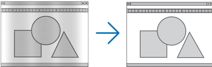
**CLOCK**..... Use this item to fine tune the computer image or to remove any vertical banding that might appear. This function adjusts the clock frequencies that eliminate the horizontal banding in the image. This adjustment may be necessary when you connect your computer for the first time.
