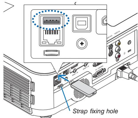
To remove the USB Wireless LAN Unit, disconnect the power cord and use the above procedure.
