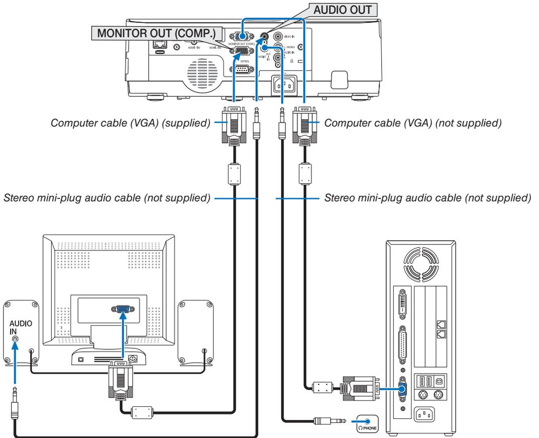
You can connect a separate, external monitor to your projector to simultaneously view on a monitor the computer analog image you're projecting.
