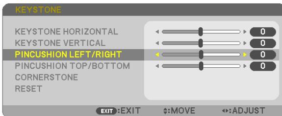
**3. Press the ◀ or ▶ button to correct distortion.**
