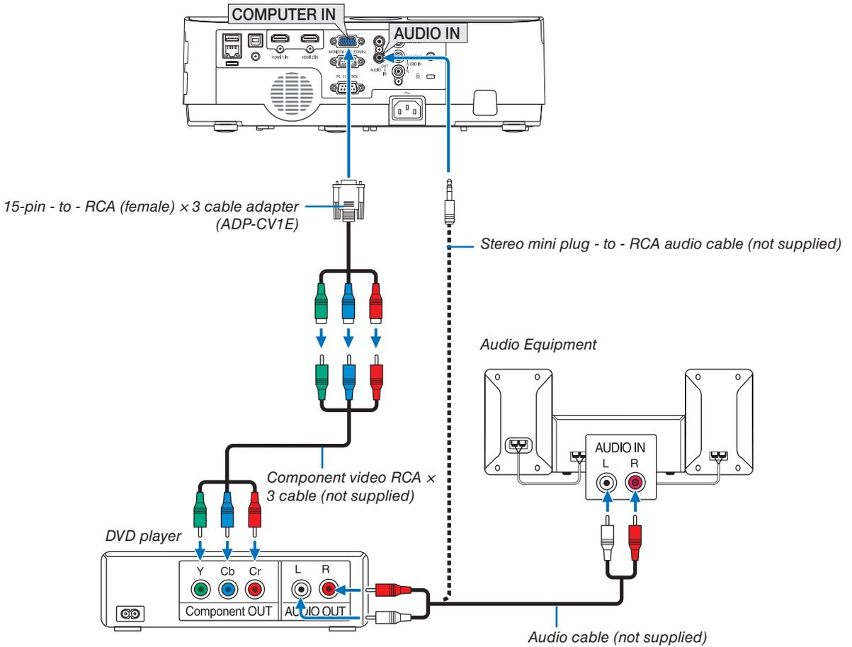
A component signal will be automatically displayed. If not, from the menu, select [SETUP] → [OPTIONS(1)] → [SIGNAL SELECT] → [COMPUTER], and then place a check mark in the Component radio button.
