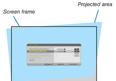
3. Align the left (or right) side of the screen with the left (or right) side of the projected image.
