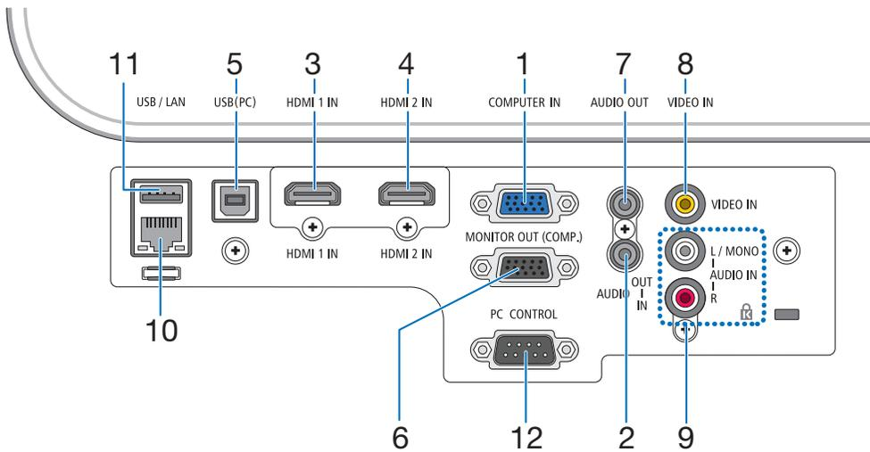
**1. COMPUTER IN/ Component Input Terminal (Mini D-Sub 15 Pin)**
