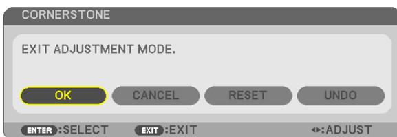
10. Press the **◀** or **▶** button to highlight the [OK] and press the **ENTER** button.
