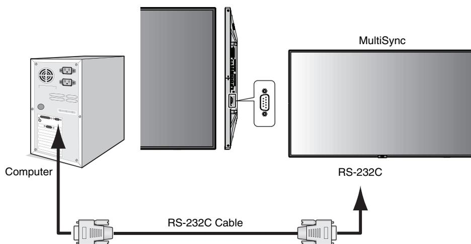
**NOTE:** If your computer is equipped only with a 25-pin serial port connector, a 25-pin serial port adapter is required. Contact your supplier for details.
