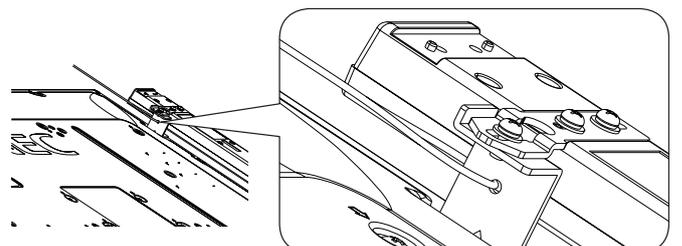
Optional speaker is installed on the side of the LCD monitor:
