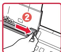
3 Load several sheets of paper with the print side facing up and slide the side paper guide against the edge of the paper stack.
