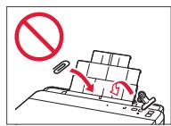
2 Open the feed slot cover and slide the right-hand side paper guide to the far right.
