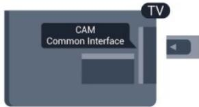
Use the Common Interface slot on the TV to insert the CAM card.
